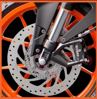
The high-tech BYBRE braking system works in perfect harmony with the advanced ABS. With a 300 mm brake disc on the front, paired with a 230 mm disc on the rear, the KTM 125 DUKE delivers exceptional pro-level stopping power.
