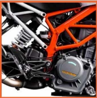
The lightweight **split-steel trellis frame** keeps the weight closer to the centre of gravity, maximizing its manoeuvrability and precision.
