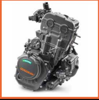
Armed with a race-bred 4-stroke single-cylinder, compact engine, this nimble yet powerful machine packs an 11 kW (14.5 PS) of peak power.
