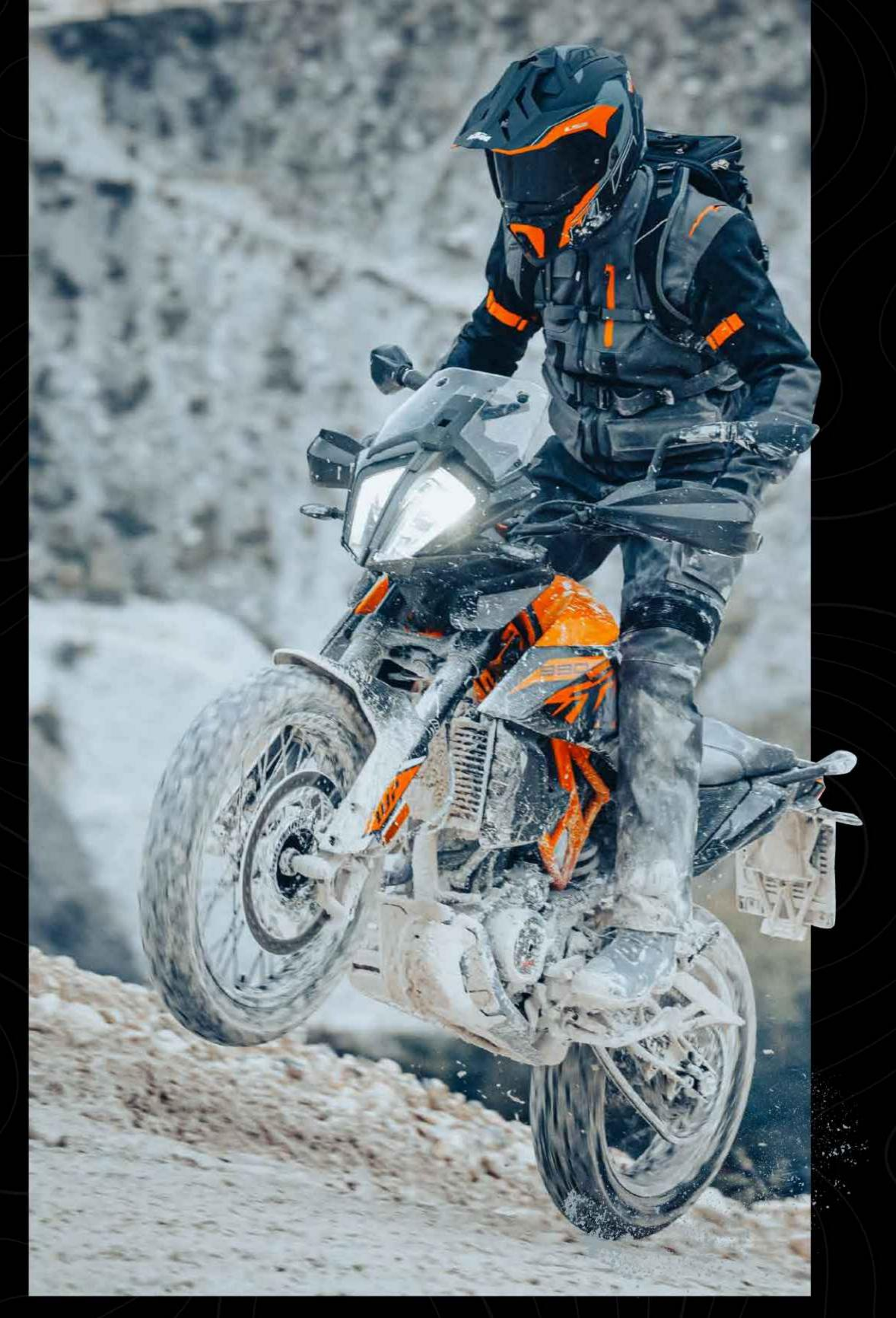
With many years of development in the toughest terrain, the 2023 KTM 390 ADVENTURE boasts WP APEX suspension at each wheel. Both the front USD and rear monoshock get an adjustable spring preload and rebound damping, it can also be fine-tuned to suit the rider, conditions, & nature of adventure. This provides a best-in-class handling package that is ready to tackle any adventure.
