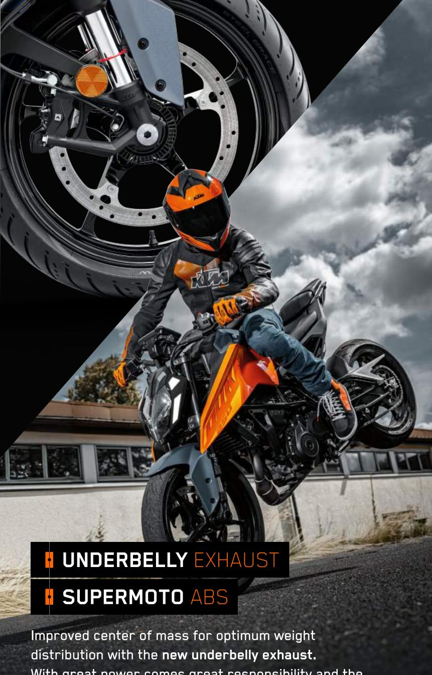
Improved center of mass for optimum weight distribution with the new underbelly exhaust. With great power comes great responsibility and the KTM 250 DUKE now comes with 320 mm brakes at the front and 240 mm brakes at the rear - whilst being SUPERMOTO ABS enabled.
