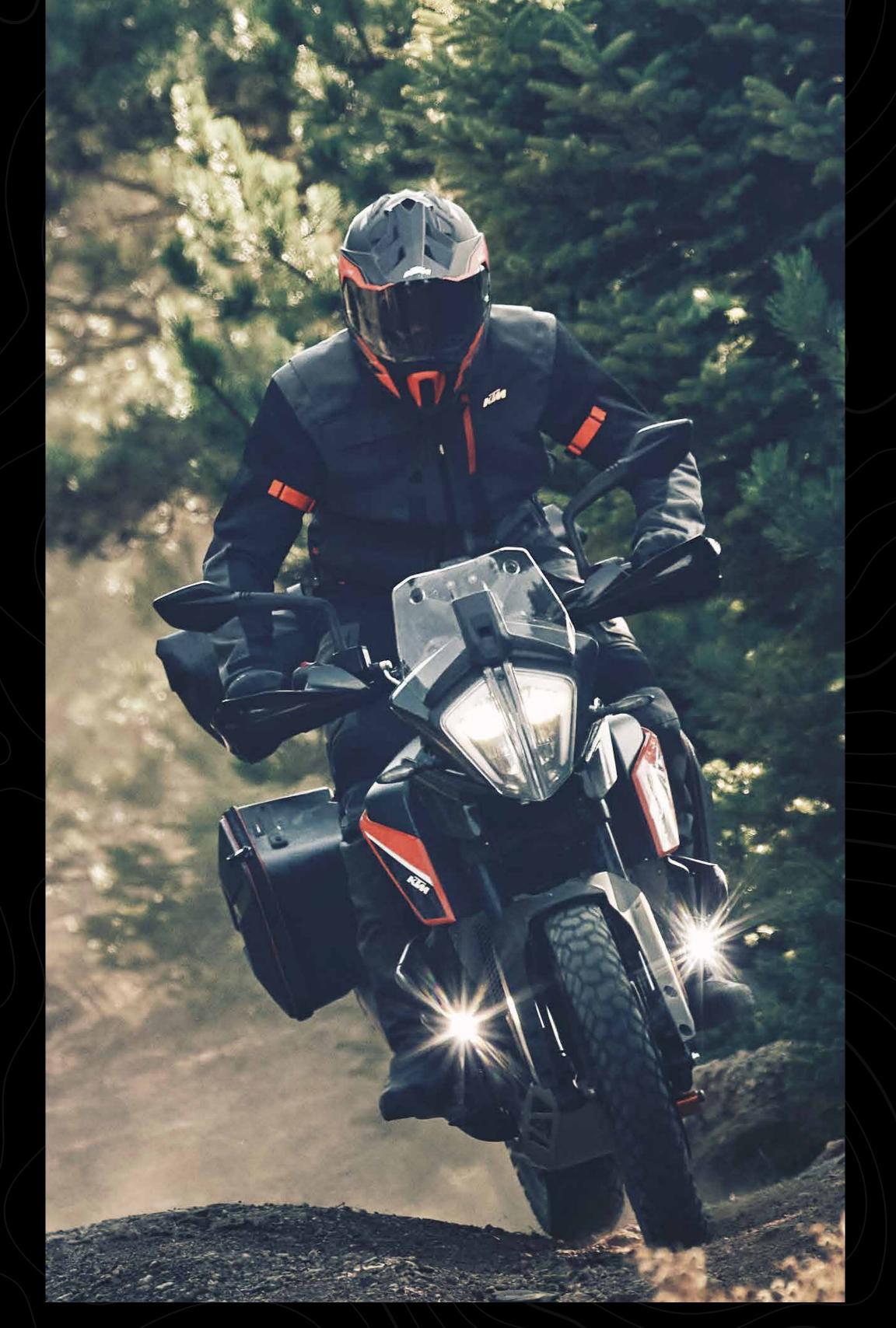
MOTORCYCLE TRACTION CONTROL (MTC) on the KTM 390 ADVENTURE is aided by 3D Intertial Measurement Unit (IMU). This LEAN-ANGLE SENSITIVE traction control system reacts when the instant rear wheel rotation speed becomes disproportionate to the riding situation and optimizes wheel spin depending on your selected ride mode.
