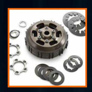
The PASC or Power Assist **Slipper Clutch** reduces rear-wheel chatter during quick downshifts so you can tame corners with ease.
