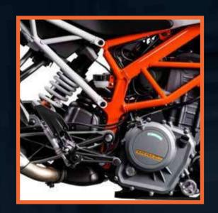
The lightweight **split-steel trellis frame** keeps the weight closer to the centre of gravity, maximizing its manoeuvrability and precision.
